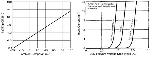
Figure 5. Typical Normalized Off-State Leakage
