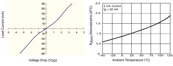
Figure 3. Typical On Characteristics
