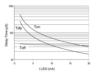
Figure 7. Typical Delay Times
