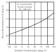
Figure 4. Typical Normalized On-Resistance
