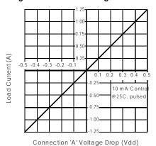
Figure 3. Linearity Characteristics
