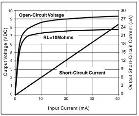
Figure 1. Typical Output Characteristics
