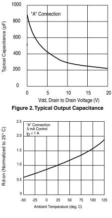
Figure 4. Typical Normalized On-Resistance
