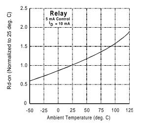
Figure 4. Typical Normalized On-Resistance
