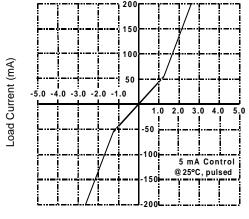
Relay's Output Voltage Drop (Vdd)
