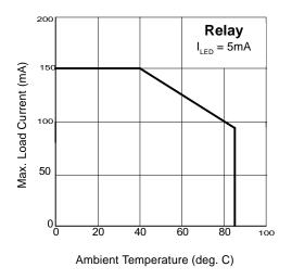
Figure 1. Current Derating Curve
