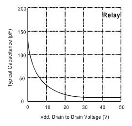
Figure 2. Typical Output Capacitance
