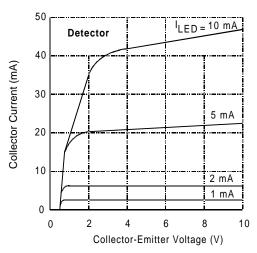
Figure 9. Typical Transfer Characteristics
