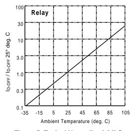
Figure 5. Typical Normalized Off-State Leakage
