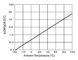
Figure 5. Typical Normalized Off-State Leakage
