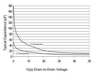
Figure 9. Typical Output Capacitance
