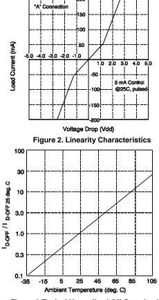
Figure 4. Typical Normalized Off-State Leakage
