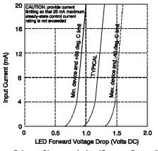
Figure 5. Input Characteristics (Current Controlled)
