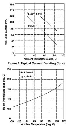
Figure 3. Typical Normalized On-Resistance
