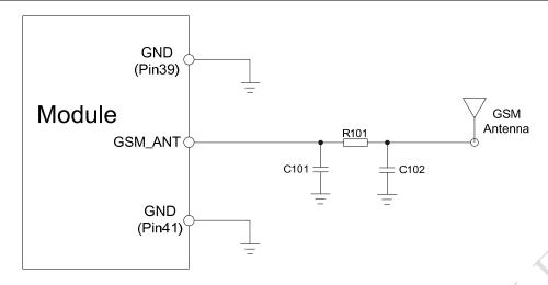
Figure 50: GSM simple antenna matching circuit
