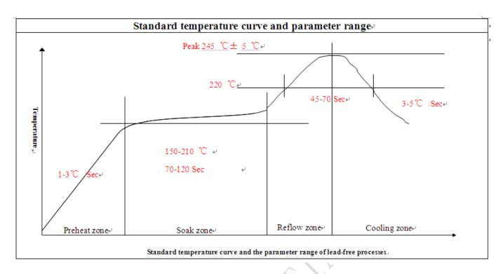
Figure 58: Typical solder reflow profile of lead-free processes
