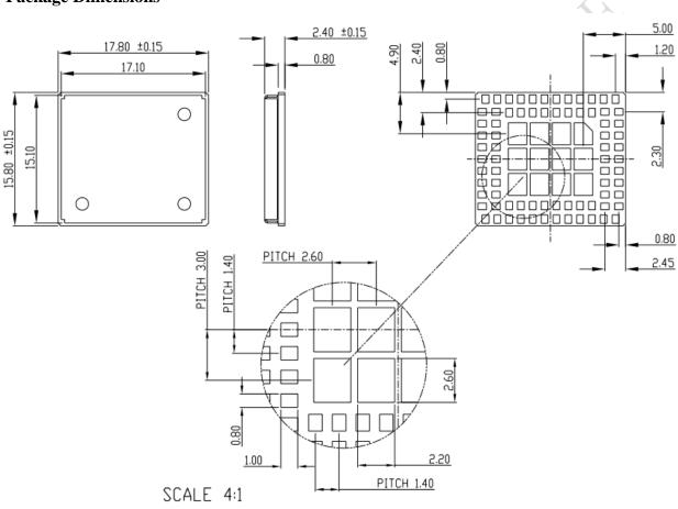
Figure 3: Dimensions of SIM800H/L (Unit: mm)
