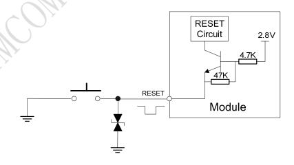
Figure 15: Reset circuit
