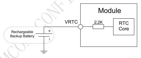
Figure 19: RTC supply from rechargeable battery
