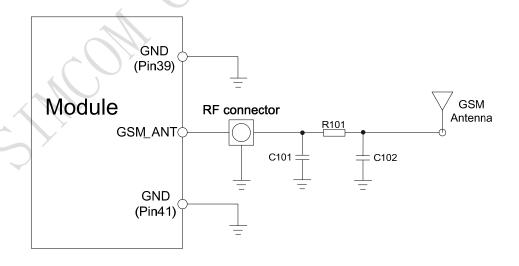
Figure 49: GSM antenna matching circuit
