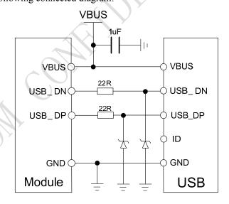
Figure 25: USB reference circuit
