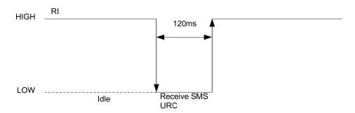
Figure 29: RI behaviour of URC or receive SMS
