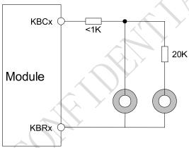
Figure 42: Keypad reference circuit
