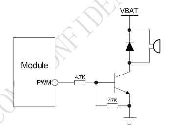
Figure 45: Reference circuit of PWM driver buzzer
