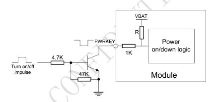
Figure 10: Powered on/down module using transistor
