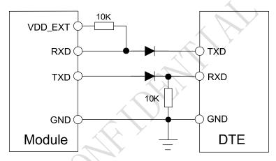
Figure 22: Diode isolation circuit
