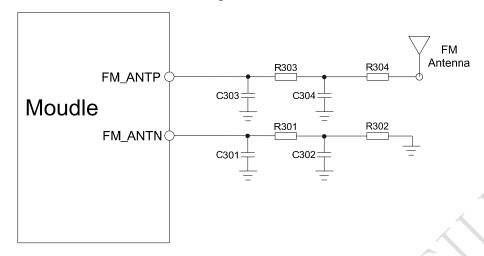
Figure 52: FM antenna matching circuit
