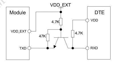
Figure 23: TX level matching circuit
