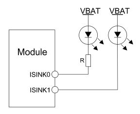
Figure 47: LED driver reference circuit
