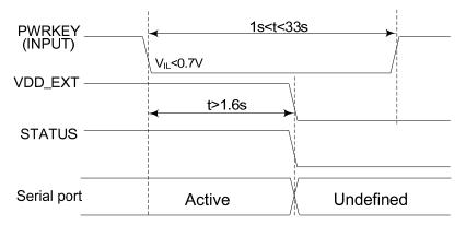
Figure 13: Timing of power down SIM800H/L by PWRKEY
