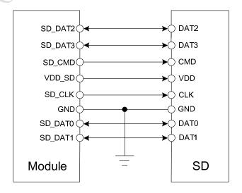
Figure 39: SD reference circuit
