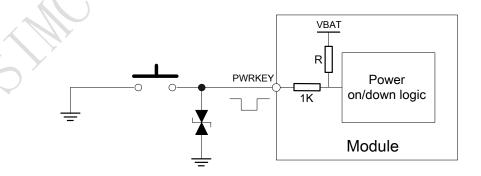
Figure 11: Powered on/down module using button
