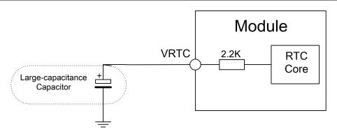
Figure 17: RTC supply from capacitor
