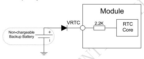
Figure 18: RTC supply from non-chargeable battery
