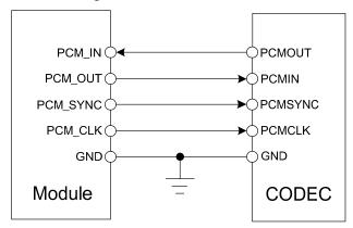
Figure 37: PCM reference circuit
