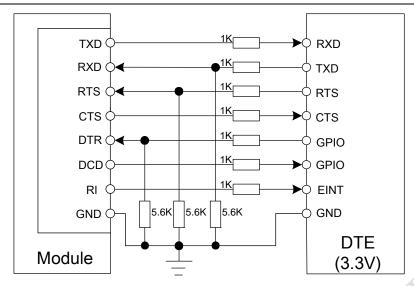
Figure 21: Resistor matching circuit
