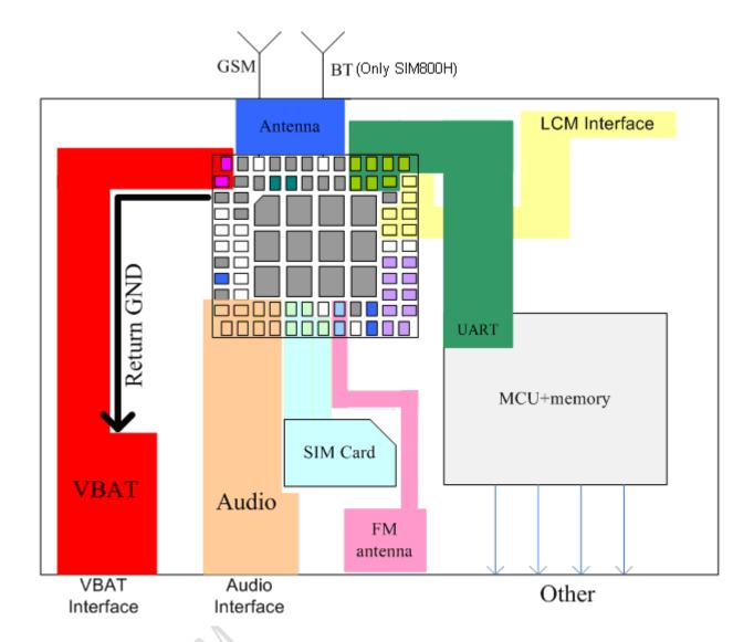
Figure 55: Recommended PCB layout
