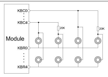
Figure 41: 50 keys reference circuit
