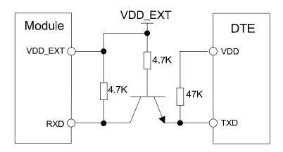
Figure 24: RX level matching circuit
