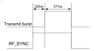
Figure 48: RF\_SYNC signal during transmit burst
