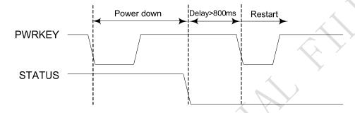
Figure 14:Timing of restart SIM800H/L
