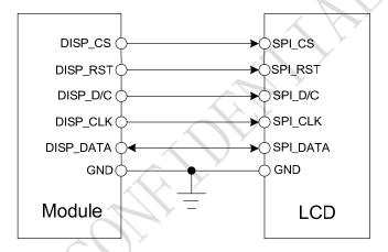
Figure 38: LCD reference circuit
