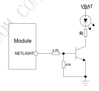
Figure 46: Reference circuit of NETLIGHT
