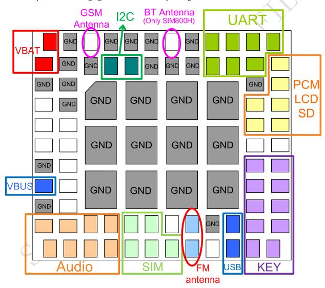
Figure 54: Pin assignment
