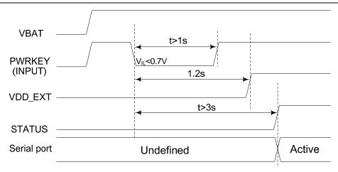
Figure 12: Timing of power on module
