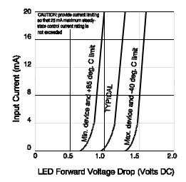
Figure 3. Input Characteristics (Current Controlled)
